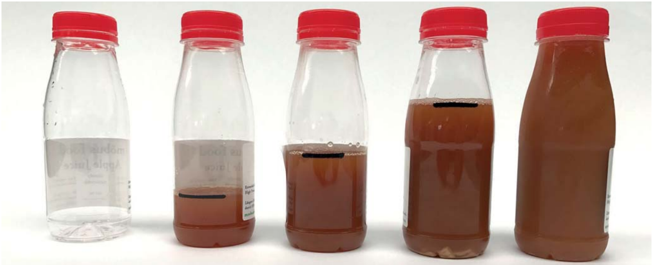
Fig. 3: The volume of air in the packaging does not affect the product in the HPP process.
