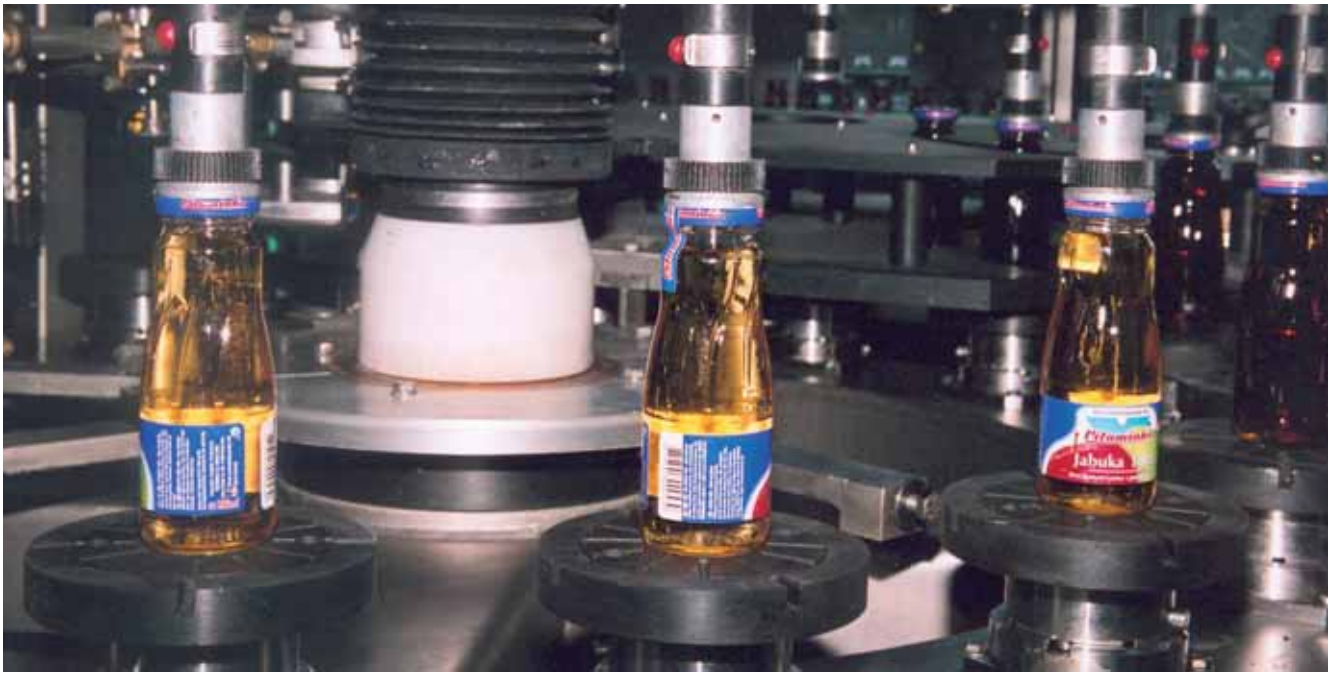
In the Innoket ROLAND 16/4, the 0.2-liter bottles receive both a body label and a tamper-evident cap label.
