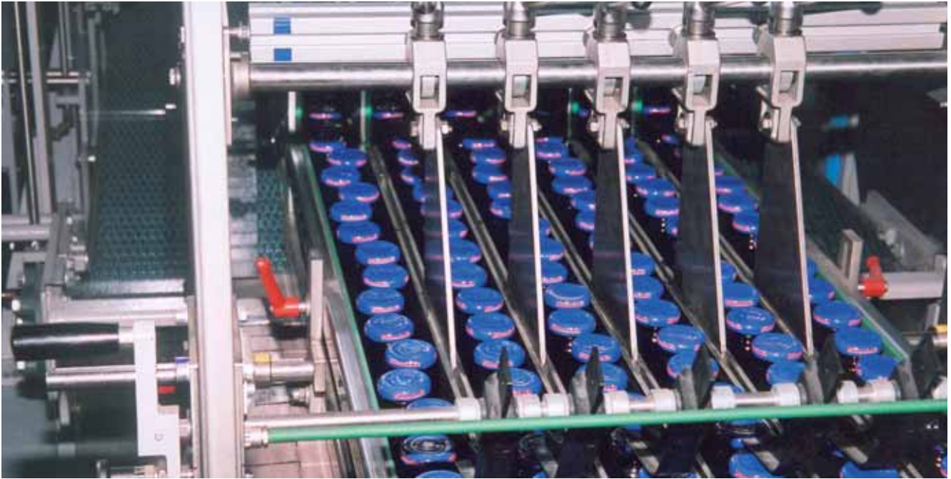
In the Innopack Kisters TSP 35 tray shrink packer, the bottles are fed into the machine according to the accumulation principle using funnel-shaped guide rails..
